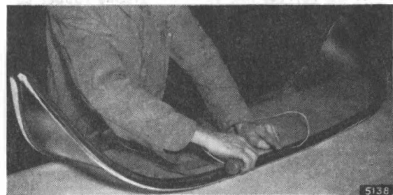
Fig. 5. Inserting cord into weatherstrip (All models)
