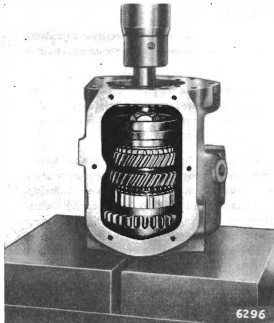
Fig. 6a. Pressing mainshaft into rear bearing
