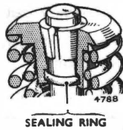
Fig. 21. Valve spring cup showing sealing ring groove
