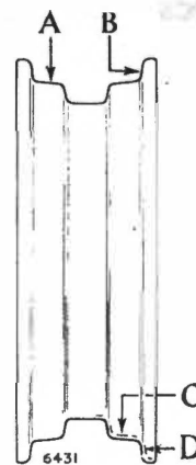
Fig. 1. Check for wheel distortion at "A" and "B" but "C" and "D" when tyre is mounted
